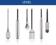
JUMO level measurement probes are used for hydrostatic filling level measurement in ventilated tanks or to determine levels in open waters. Differential pressure transmitters are used for pressurized filling level measurement in closed tanks.
