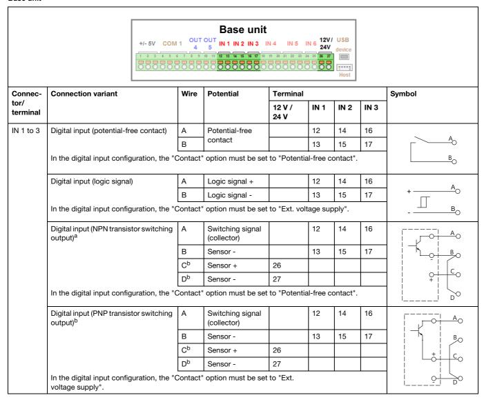
The connection variants for transistor switching outputs (NPN / PNP) are especially important for the flow measurement via impeller sensor (type 406020, parts no. 00525530, 00525531) at inputs IN 2 and IN 3 (pulse frequency inputs). However, alternative sensors with transistor switching output can also be connected.
