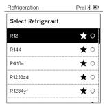
6.2 Setting the refrigerant: Press [▲] or [▼] to select the refrigerant and press [Menu/Enter] to confirm.
